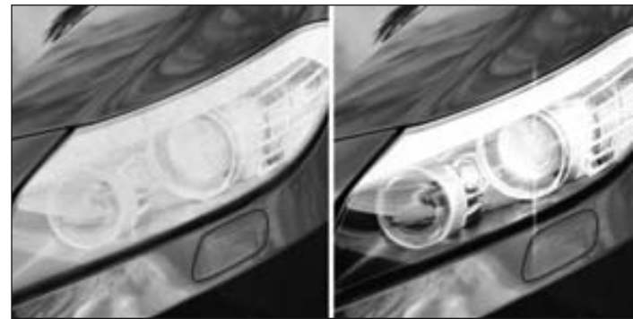
A cloudy headlight lens (left) before restoration and (right) a headlight lens restored to "like new" condition with an available restoration kit.
